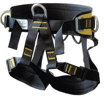
Belt fitted with ergonomically profiled padding, connecting and adjusting buckle, side attachment buckles and attachment point for work in a harness. Work positioning belt / sit harness PB 70 complements fall protection equipment and prevents falls from height during works at poles, trees, building structures, etc.
