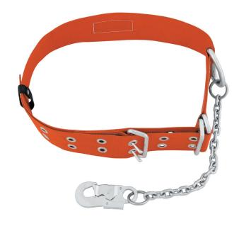
Work positioning belt PB 60 is made from a single polyester webbing strip connected by an aluminium buckle. Fitted with a welt to enable smooth belt length adjustment (length between 0.45m and 2.0m). Chain with steel connector AZ 002 at the end. Work positioning belt PB 60 complements fall protection equipment and prevents falls during works at height.
