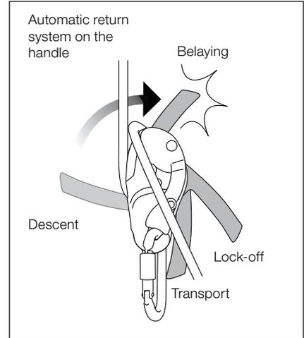
The RIG descender's multi-functional handle allows the user to control the descent and to position himself at the work station. The automatic return system on the handle limits risks in case of an involuntary action by the user.
