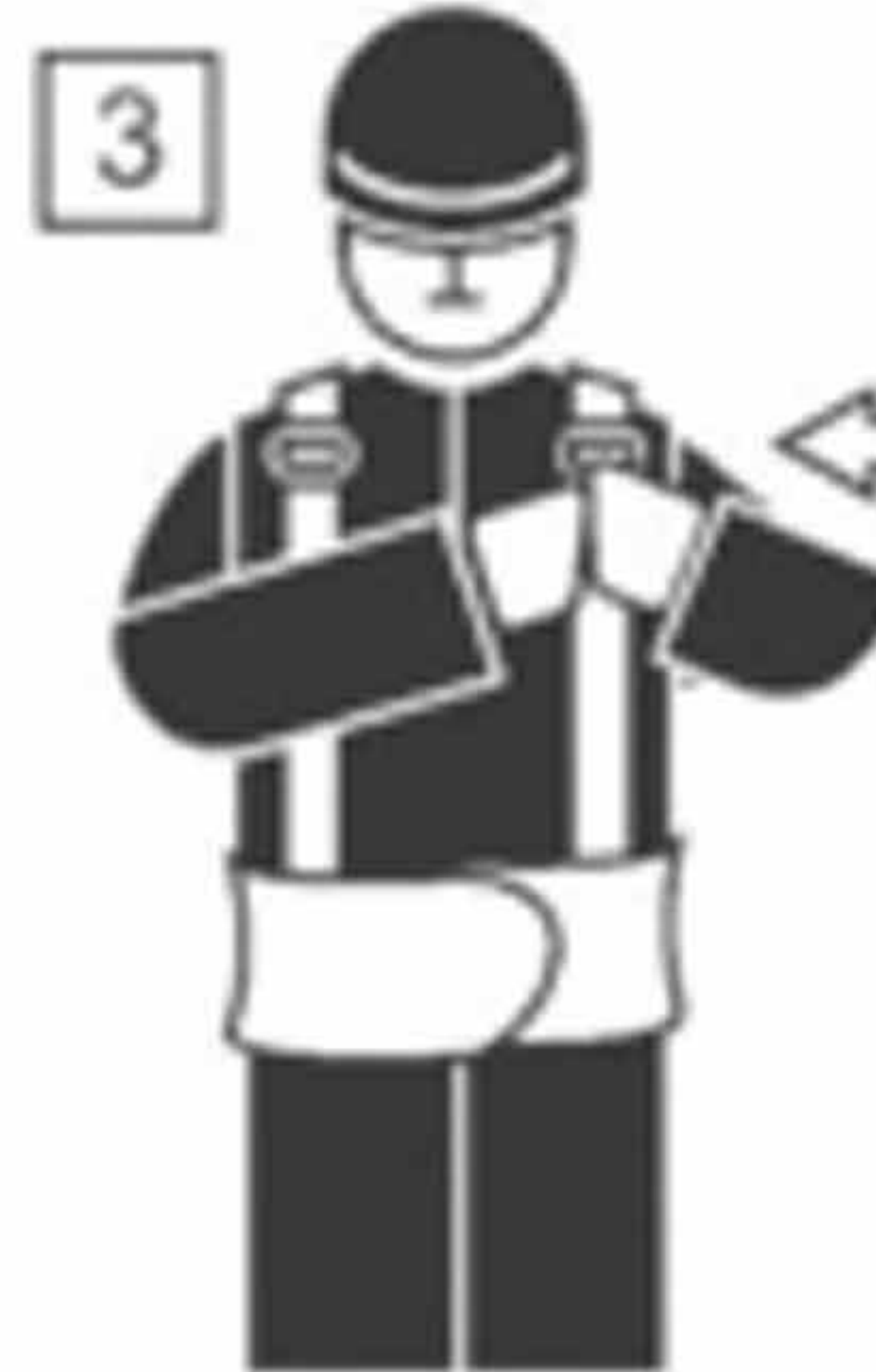
3 Adjust the belt position with the use of the adjustment buckles on the shoulder straps.
