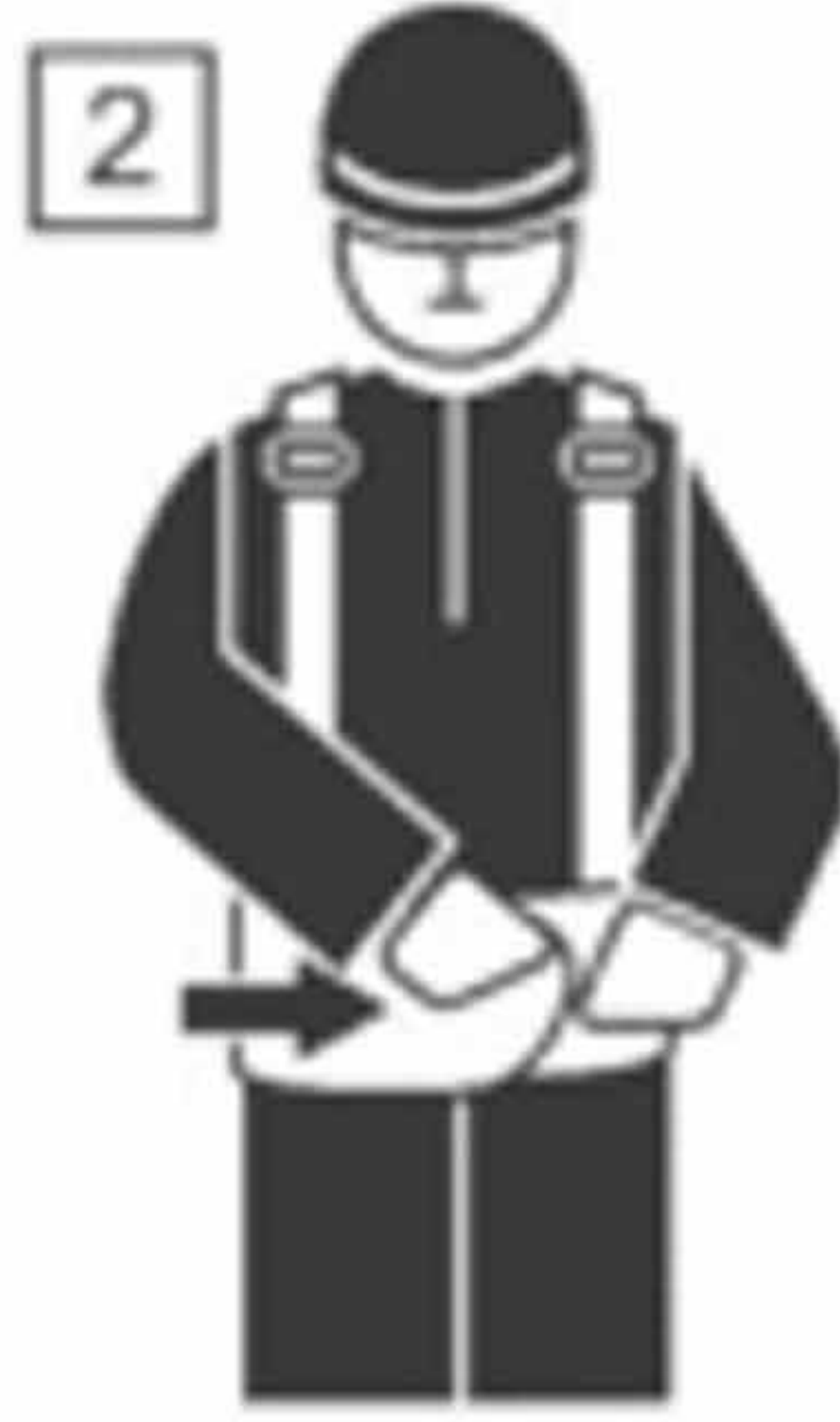
2 Tighten the belt and fasten the Velcro, placing the right hand end of the belt over the left hand end.
